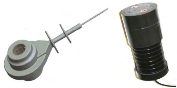
Fig. 23: Two different prototypes of integrated voltage and current sensors
